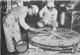
THE MAGNAFLUX operation is carried on in an area outside the EIG lab which is adjacent to the metal trades location. The convenience of the lab's new location presents itself when heavy pieces in the main shops need special EIG attention.
